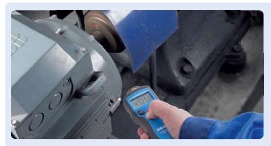
The laser optical system allows easy and quick measurements at a safe distance from rotating machinery.
